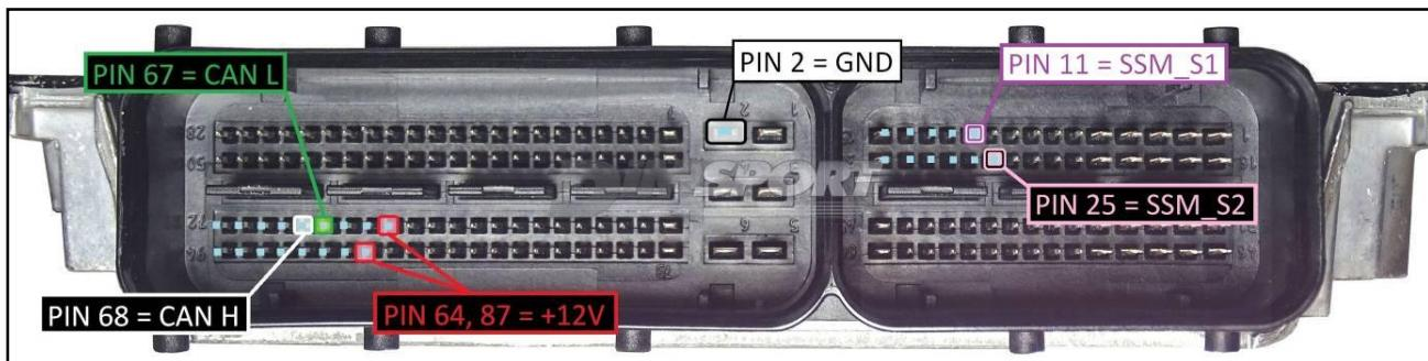
After the correct reading of the password you can open the ECU and perform the connections for the BOOT mode.
