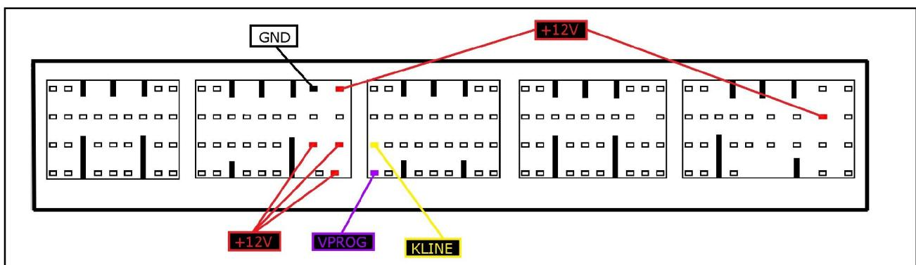
To the 5 power feeding pins you can connect both wires red and orange, they both have 12 Volt signal.
