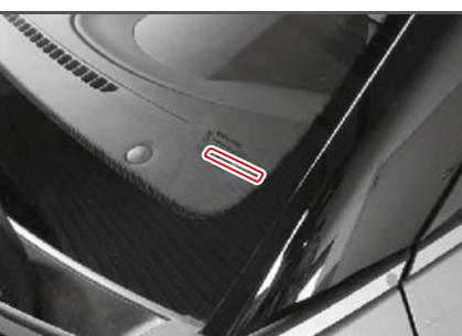
Visual VIN label is located on the driver's side instrument panel.
