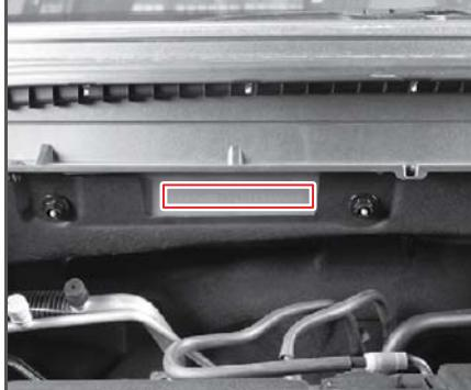
The VIN number is stamped on the passenger side fire wall.
