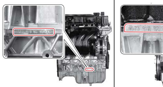
**Gasoline engine:** The engine number is stamped lower area of cylinder block in intake manifold side.
