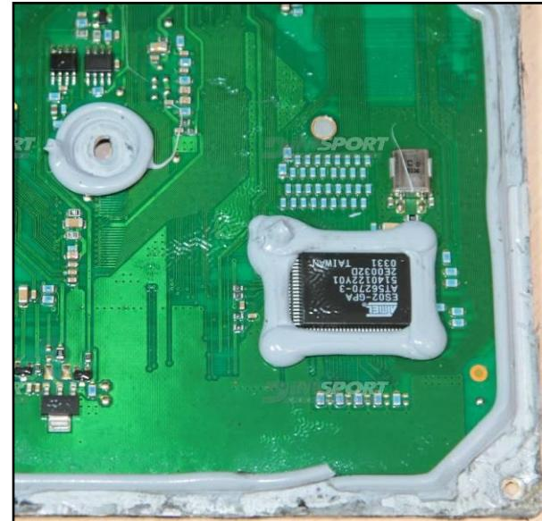
In order to perform the BDM reading it is necessary to make a little bridge on the quartz as shown in the following picture. Remove the bridge from the quartz at the end of the procedure or before restoring the ECU on the vehicle.
